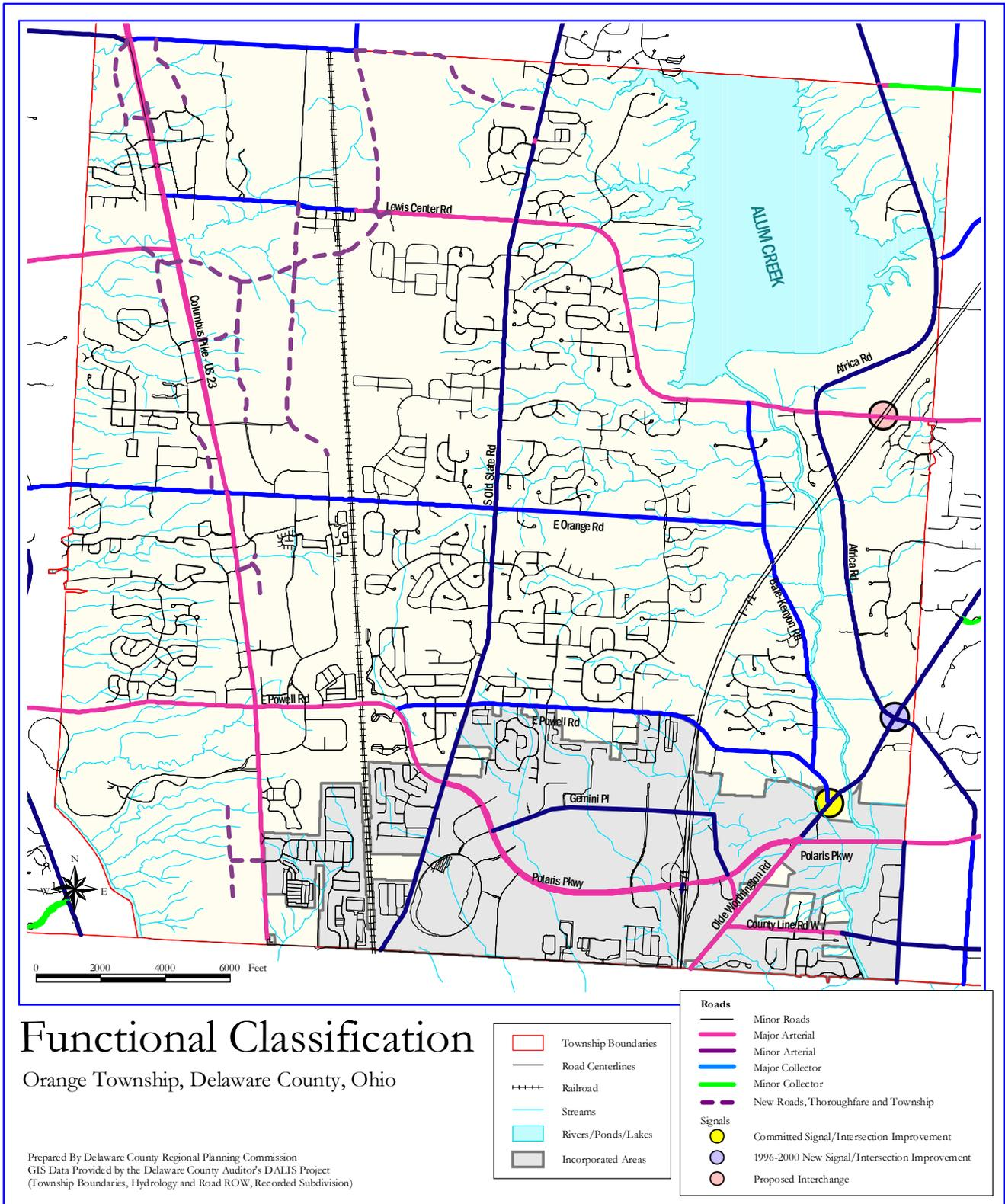
Arterial roads have the primary purpose of carrying through traffic to and from residential, commercial, and industrial areas and the secondary purpose of providing access to abutting property. They are usually a continuous route carrying heavy loads and Average Daily Traffic (ADT) in excess of 3,500 vehicles.
